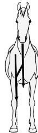
Fig.3. The centre of gravity results in a greater force being applied to the medial side of the leg and hoof wall. After 'Shoeing for Performance', by Price & Fisher.
